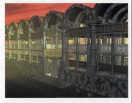
the effect of forcing the voussoirs [wedge shaped blocks—S.S.] together instead of apart... Arches may rest upon light supports [i.e., relatively light — S.S.]. However, where they occur in a row, because the thrust of one arch counteracts the thrust of its neighbours, the system remains stable as long as the arches at either end of the row are buttressed. This system is put to use in such structures as arched stone bridges and ancient Roman aqueducts".
